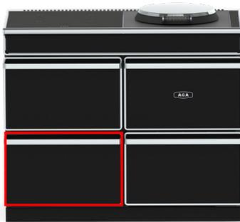
The fan oven is heated by an element in the back of the oven and hot air is distributed around the cavity by a fan. This allows for a faster heat up time and the flexibility of a range of cooking temperatures; B1-B4 for baking and R6-R9 for roasting.
