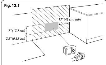
The dimensions shown are correct when the range is set to its lowest position
