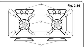
A - Broiler elements, B - Convection element, C - Base heat elements
