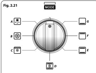
A – Thaw & serve, B – Convection oven, C – Convection broiling, D – Fan assisted oven, E – Conventional oven, F – Browning element, G – Warming,
