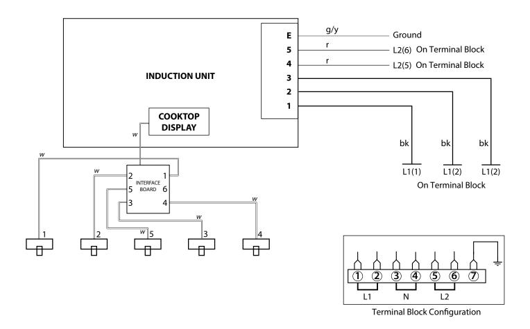
**Key**The connections shown in the circuit diagram are for single-phase. The ratings are for 240V, 60Hz
