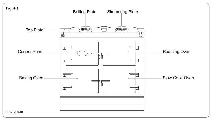
The AGA DC3G has the traditional cast iron ovens with independently controlled hotplates.
