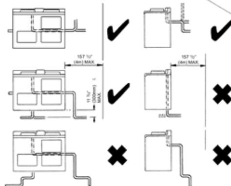
DOWNWARD RUNS UP TO 11 1/4" (300mm) BELOW THE APPLIANCE ARE ALLOWED, PROVIDED ONLY ONE BEND IS USED.
